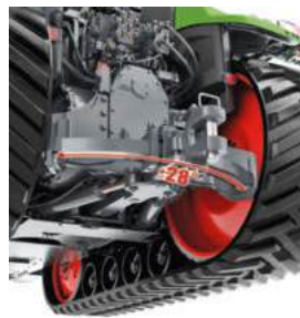
Swivel drawbar The drawbar can be swivelled 28° to the left and right.
