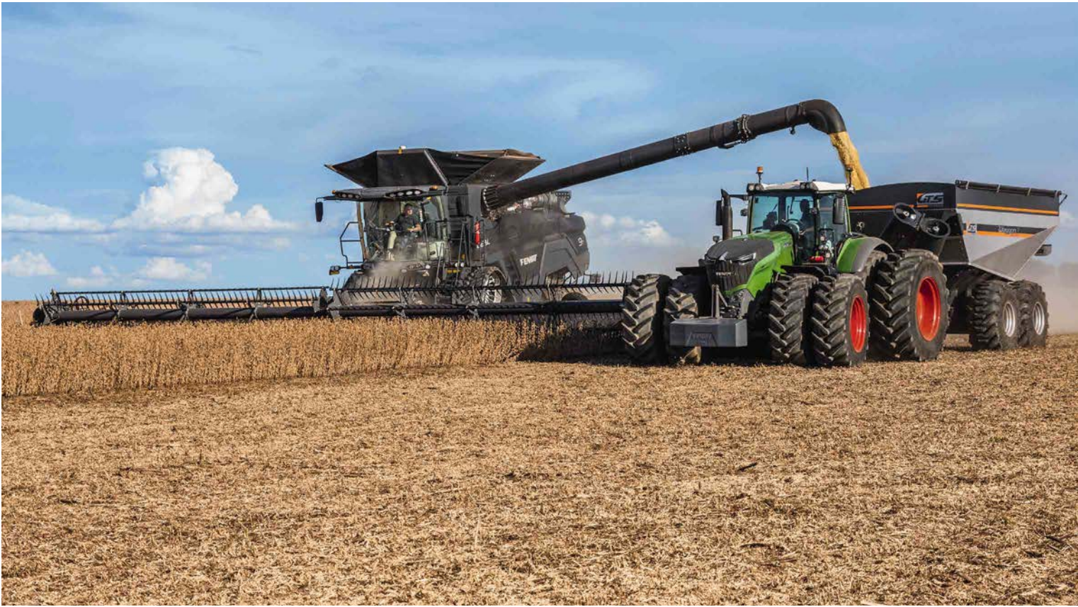
Fewer and shorter stops for unloading are soon reflected in a greater daily yield – sensors for yield and moisture and a grain quality camera are fitted to the elevator. The data is accurate to 98%, and applied with the VarioDoc ISOBUS standard, live yield mapping and IDEALharvest™.
