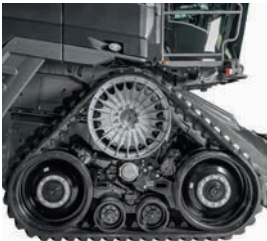
The TrakRide crawler drive minimises ground pressure.
