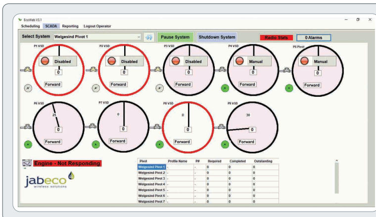
Figure 1: SCADA Display of a Pivot Control system
